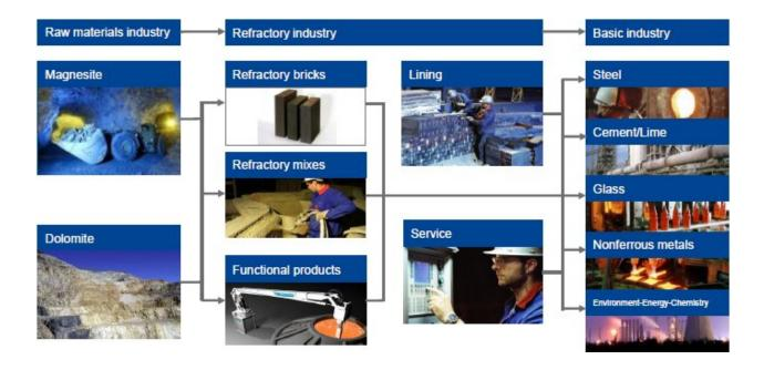
Refractories are used either where high temperature or high rate of abrasion/corrosion/erosion is involved. Traditionally, refractories are made of naturally occurring minerals such as bauxite, kyanite, magnesite, fireclay, chrome ore etc. Lately, however, the industry has been using man-made raw materials such as brown-fused alumina, tabular alumina, fused magnesia, silicon carbide, magnesia alumina etc.
